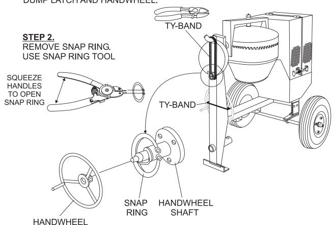
PLACE HANDWHEEL ONTO HANDWHEEL-SHAFT.
